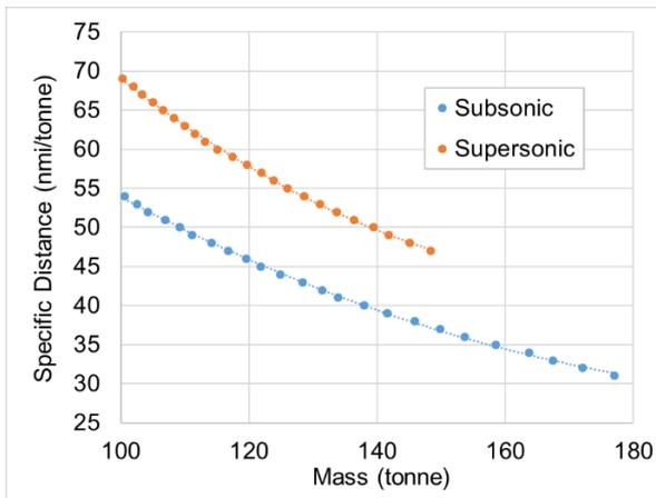
Figure 2. Specific distance vs. instantaneous mass for Concorde's optimal cruise condition
