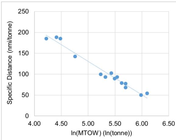
Figure 1. Specific distance vs.  $\ln(MTOW)$  for airliners serving medium-haul routes
